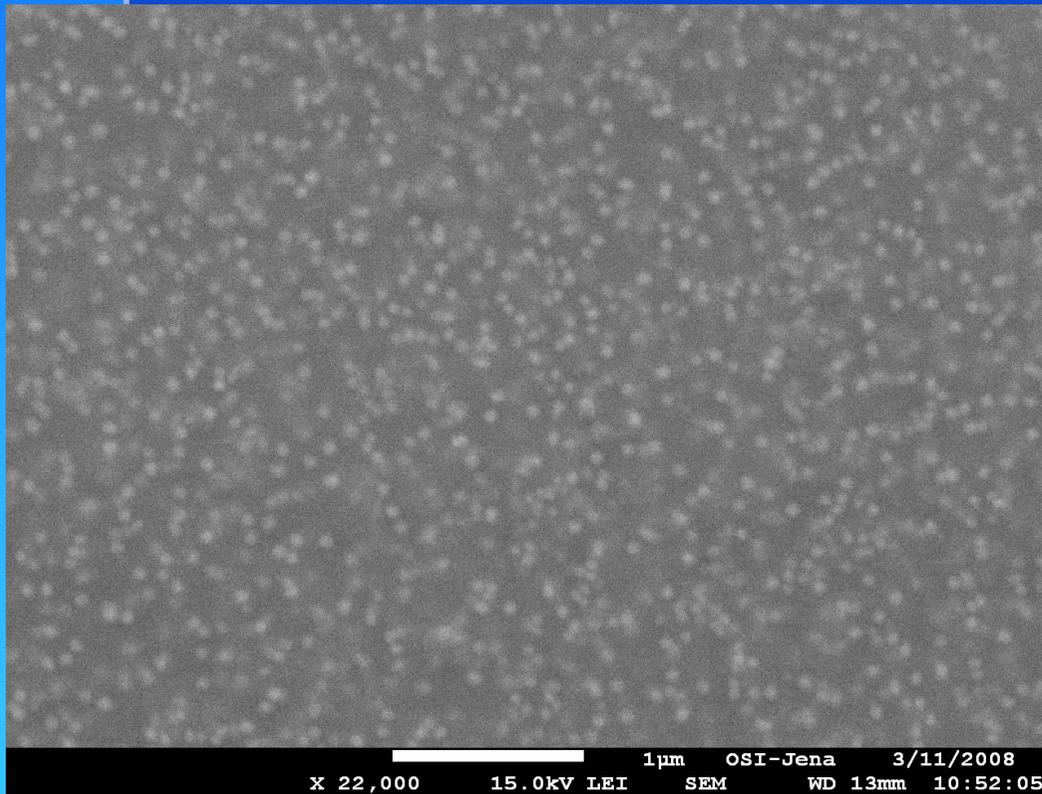
SEM (SE) image of C-covered sample with 15 mol%  $\text{Fe}_2\text{O}_{3-y}$  and 8,5 mol%  $\text{MnO}$ , annealed for 3h at 550°C.
