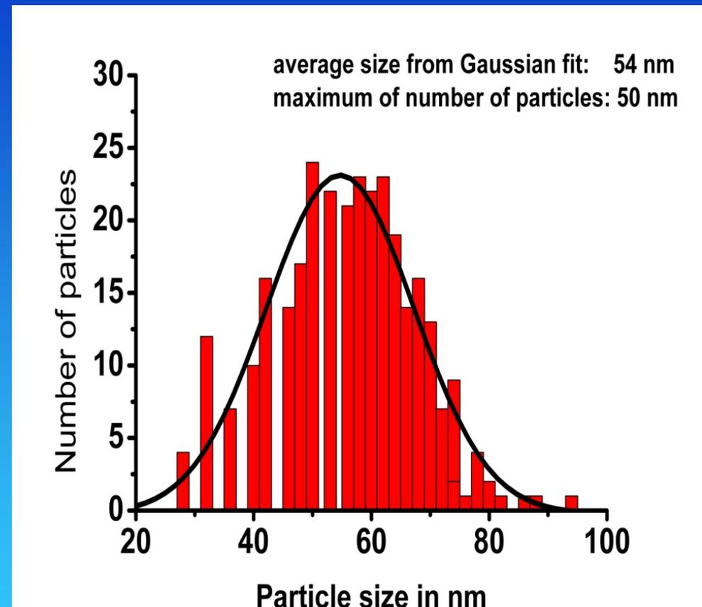
Particle size distribution for a sample annealed at 550° for 3 h.
