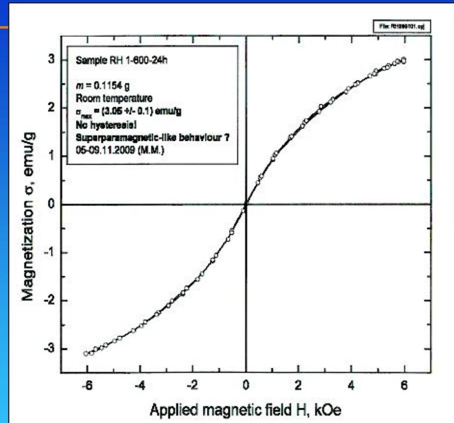
Magnetization vs. external magnetic field for a sample with 15 mol%  $\text{Fe}_2\text{O}_{3-y}$  annealed at  $600^\circ\text{C}$  for 24 h.
