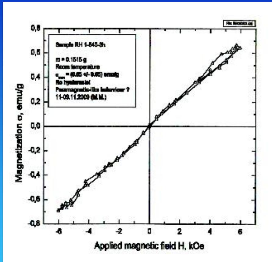
Magnetization vs. external magnetic field for a sample with 15 mol%  $\text{Fe}_2\text{O}_{3-y}$  annealed at  $540^\circ\text{C}$  for 3 h.
