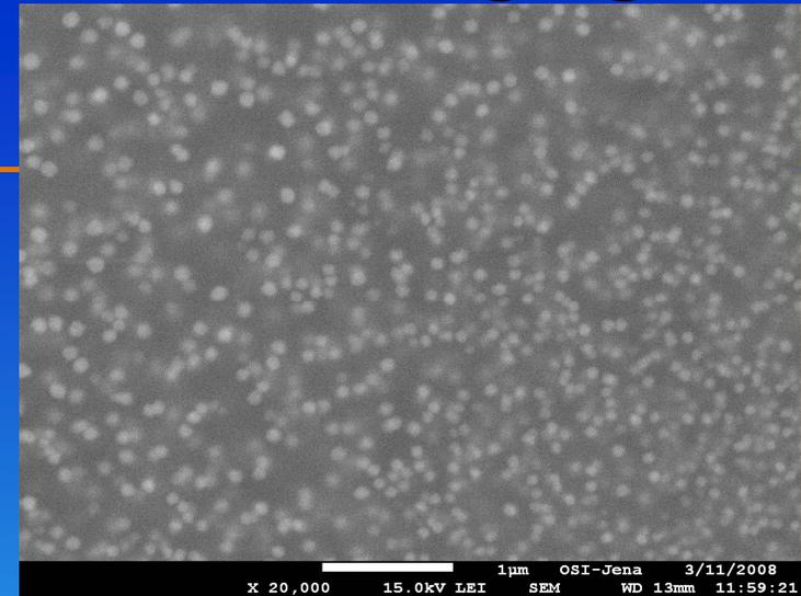
SEM (SE) image of C-covered sample with 15 mol% Fe<sub>2</sub>O<sub>3-y</sub> crystallized for 10 h at 550°C.
