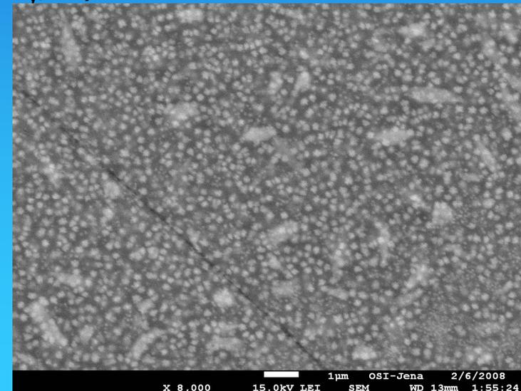
SEM (SE) image of C-covered sample with 15 mol% Fe<sub>2</sub>O<sub>3-y</sub> annealed for 24 h at 600°C.
